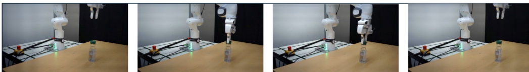
(d) Opening a Bottle Cap: A delicate task that demands precise rotation and grasping control.
