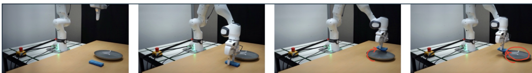
(c) Wiping the Plate: This task involves covering the majority of the surface area of the plate uniformly. It requires planning the path for the sponge to ensure most of the plate is cleaned.
